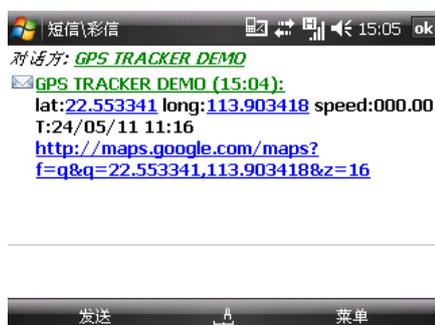
Tracking location , When no GPS signal, the SMS includes the last valid
