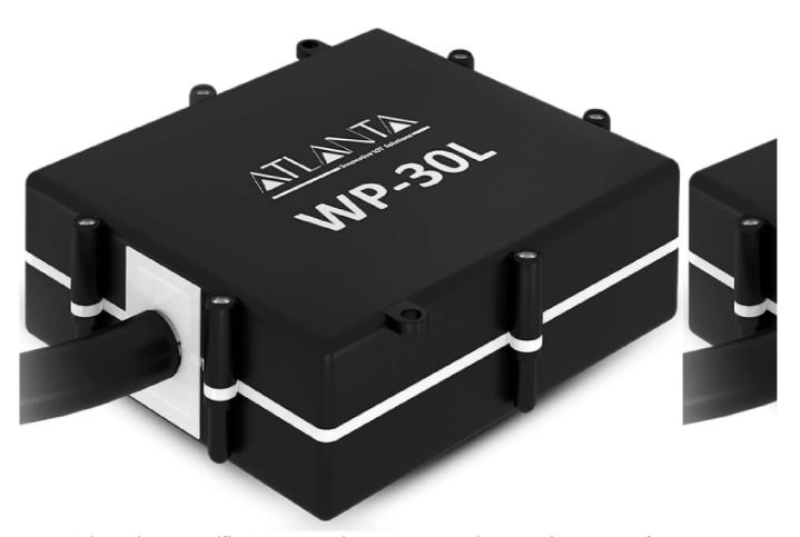
WP-30L is an iCAT certified tracker with GNSS, meeting requirements of GAGAN support, 3 servers functionality, internal battery, accelerometer and gyroscope, Embedded SIM, tamper-proof (IP67 rating), and powerful WEB FOTA to fulfill firmware updates requirement.
