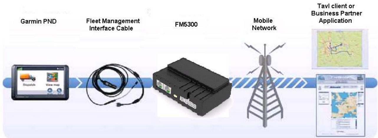
Figure 68 FM53+Garmin operational scheme
